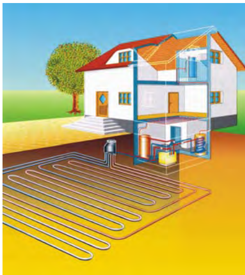
Fig. 8.28 Horizontal Earth coupled heat exchanger system (after [1999Ano a ]; yellow box in building basement: heat pump).
