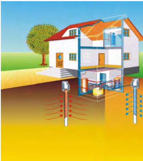
Fig. 8.32 Groundwater heat pump system (after [1999Ano a ]; yellow box in building basement: heat pump).
